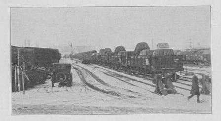
The Boston Terminal is equipped with a derrick propelled by its own power, and especially adapted to unload this class of traffic. Immediately upon arrival of these trains, the cars were placed in such a manner that this derrick could work on an adjoining track and lift the cars off and place them on the ground. It is possible to unload an automobile a minute and the operation is only restricted to the ability of the consignee to remove them. This train was actually unloaded in one day.
